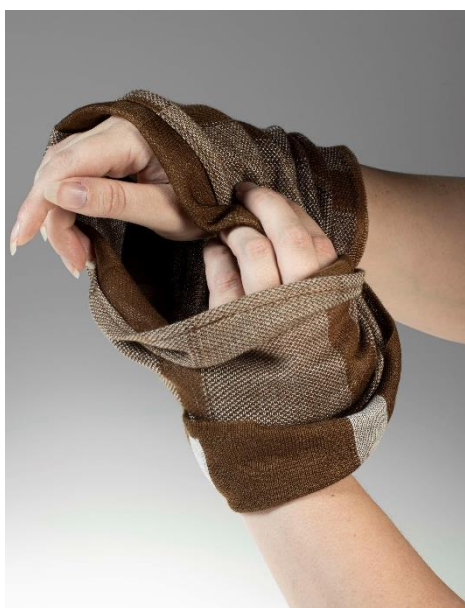
Lignin yarn prototype from Cellumimicry project. Photo by Anne Klennunen
