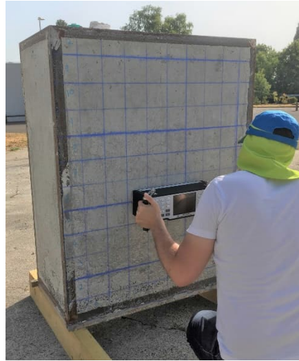
Figure 1. Acquisitions on one of the mock-ups with an ultrasound tomograph
