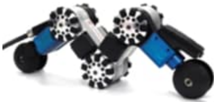
Figure 18. AIRo-5.1 snake robot [22]
