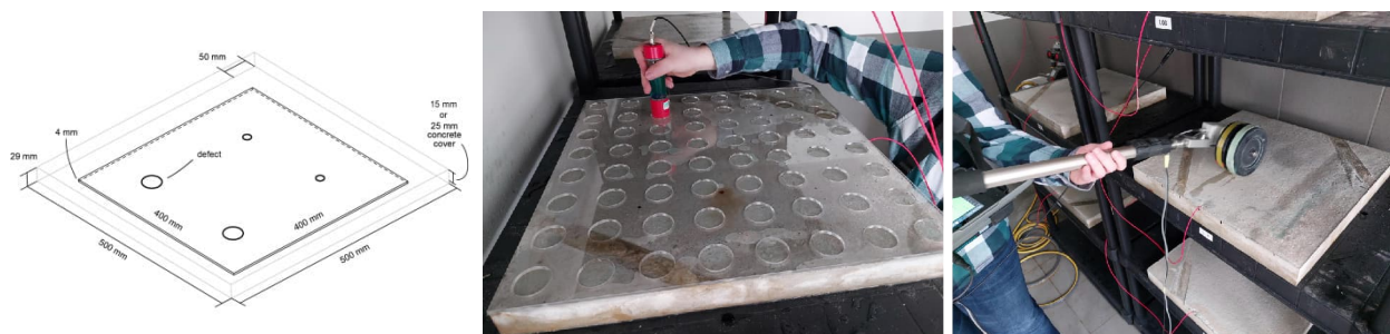
Figure 1. Sketch of the specimen (left), PM measurements with rod electrode (middle) and 1-wheel electrode (right) on the mock-up specimen.
