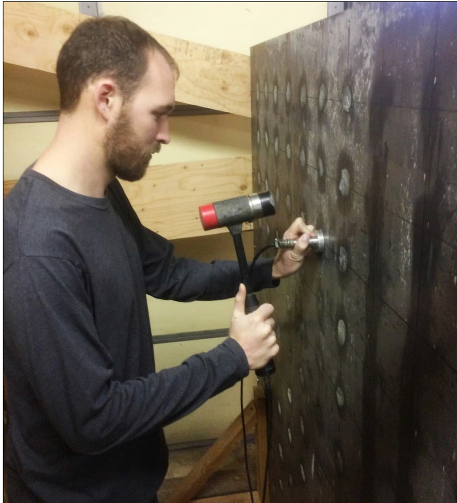
Figure 8: SIR Testing with 3-lb impulse hammer and Wilcoxon velocity transducer on Wall #1.
