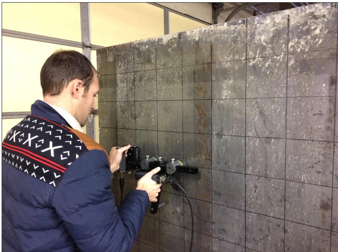
Figure 14: Spectral Analysis of Surface Waves (SASW) Testing on Wall #1 (Horizontal Test Direction) with SASW-S bar with 2 displacement transducers and IE-1 solenoid impact source at left end of bar.
