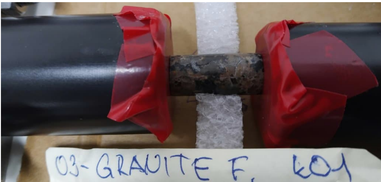
Figure 14. Granite rock cylinder squeezed by two ultrasonic transducers 150 kHz (P-wave)
