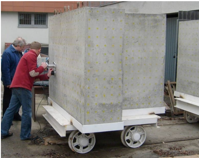
Figure 5. Photo of the massive concrete blocks at BUT [9] (left). Drawing of the block with artificial honeycombs (H), ducts (V) and rebars [11] (right).
