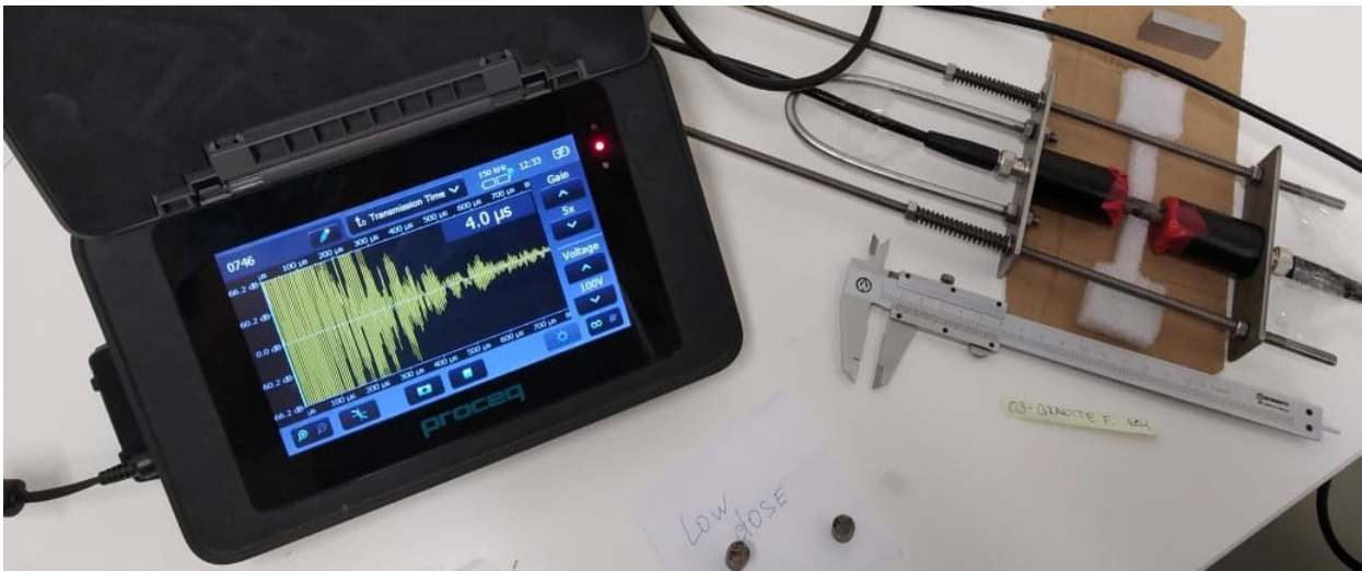
Figure 13. Ultrasonic pulse measurement by Pundit PL200 before the irradiation
