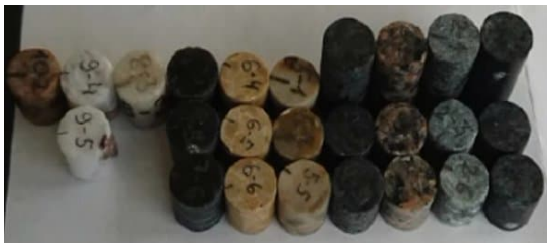
Figure 2. Fabricated cylindrical samples (10 x 10 mm)
