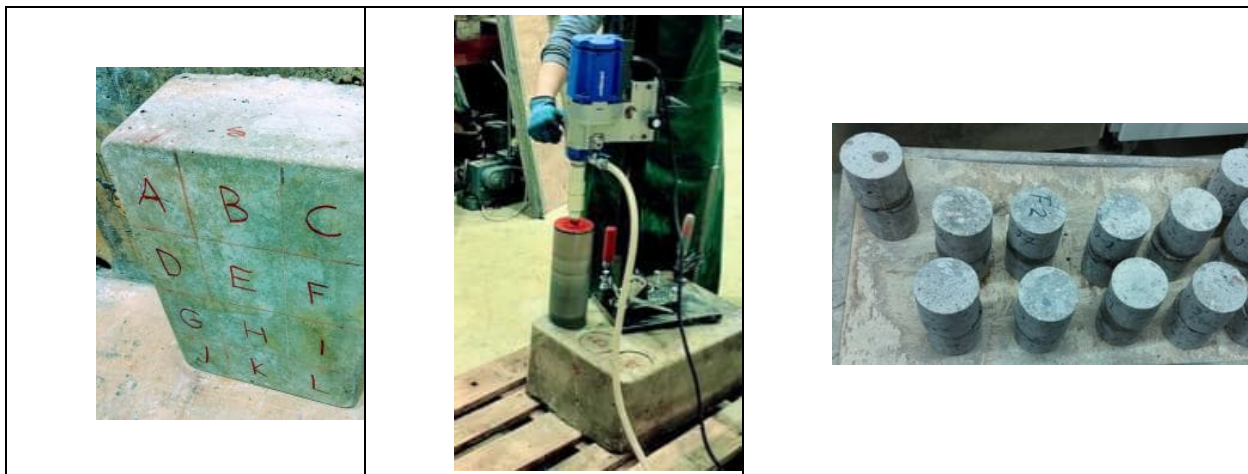
Figure 4. Drilling of core from the concrete slab cast of the concrete used in the wall concrete and stored in the same condition.
