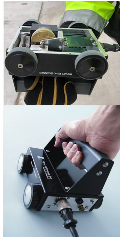
Figure 3: Impact Echo Scanning (IES) on steel side of Wall #1 and view of underside of IES unit with rolling displacement transducer on spring and normal and large solenoid impactors for tests every 1 inch (25.4 mm) and a close-up view of the IES unit.
