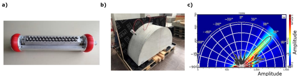
Figure 6. Ultrasonic borehole probe: a) phased array probe, b) specimen to test directivity, c) measurement results (grey scale) for 45° focussed beam overlain on respective beam simulation (colour plot).
