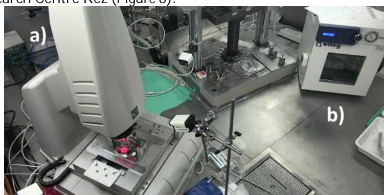
Figure 6. a) Vertex 251HM and b) furnace in hot cell
