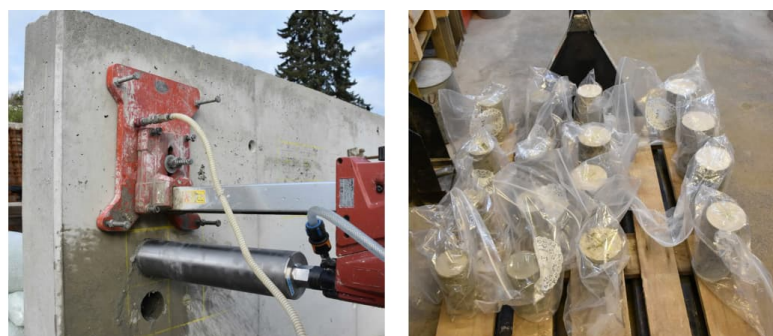
Figure 4. Drilling of the concrete cores. (a) Drilling setup and (b) specimens sealed with plastic bags after coring.
