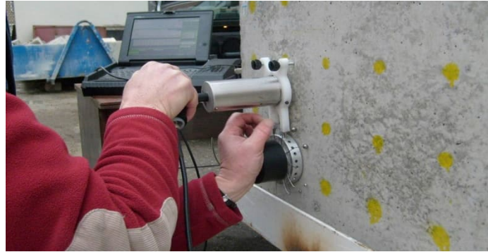
Figure 14. Impact-echo measurement of the front wall of block with artificial objects in Brno [9].
