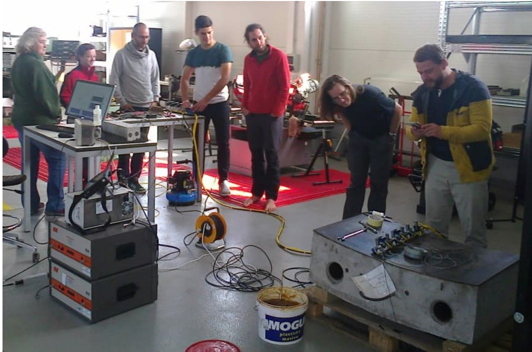
Figure 1. The mock-up of angular section of concrete biological shield with two holes inside
