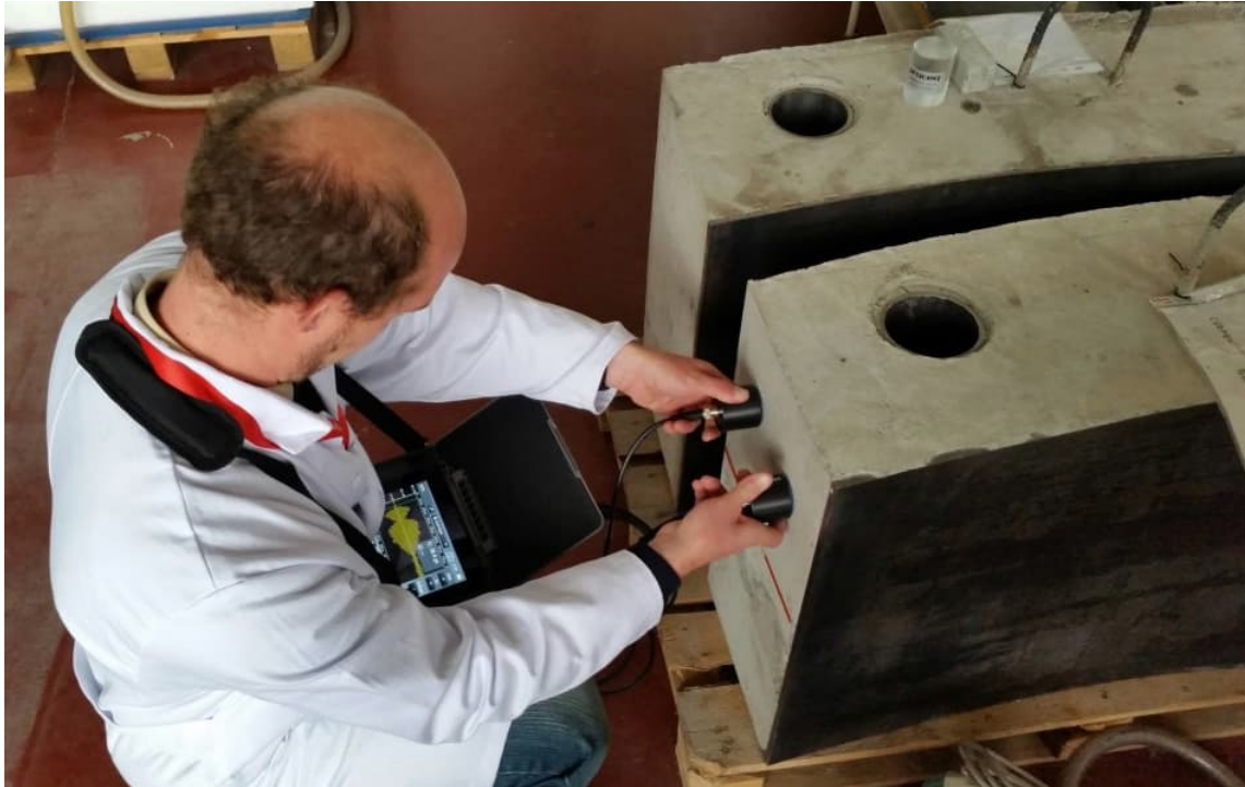
Figure 7. Indirect ultrasonic pulse testing of RPV cavity mock-ups using PUNDIT PL200 instrument
