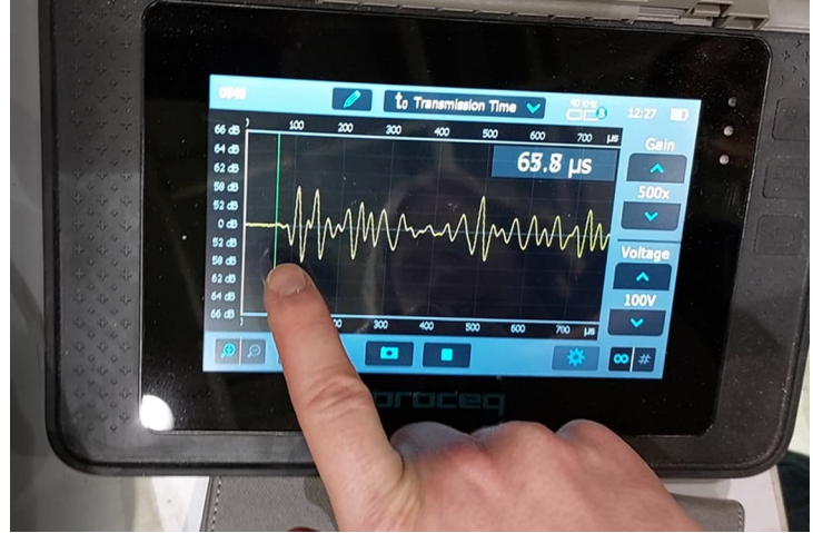
Figure 4. Views of a chamfered cube specimen and the first time arrival determination
