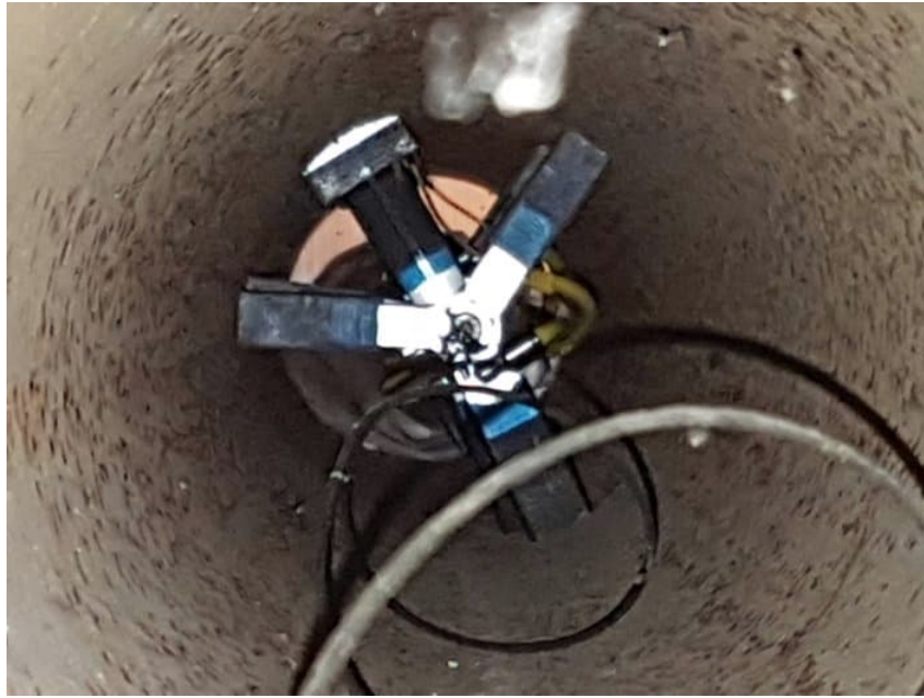
Figure 11. Manipulator Horymir during NDT inspection of Greifswald NPP RPV cavity
