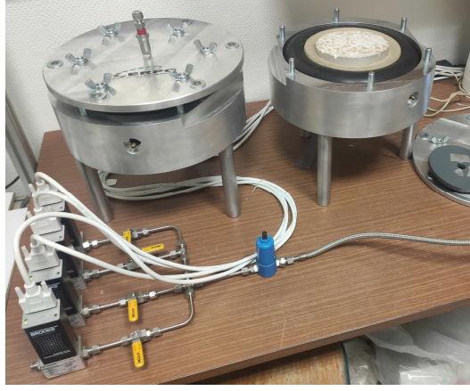
Figure 1. Cembureau apparatus for concrete permeability measurement in laboratory
