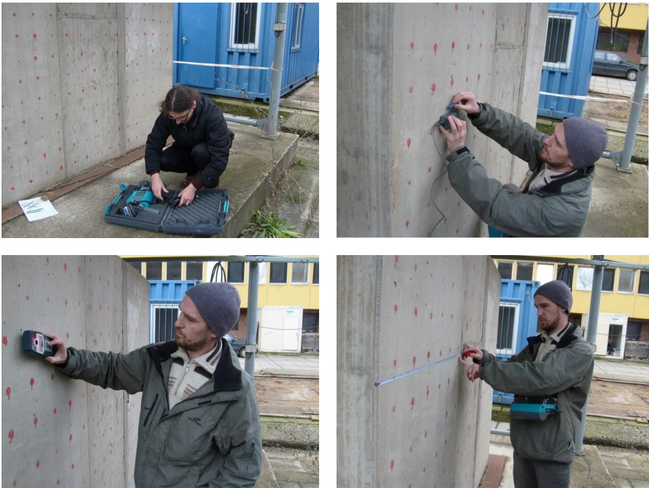
Figure 13. Locating the steel bars in block No. 5 in Rez with the Profometer 5 (right a bottom) and with the blue Bosh (top left).
