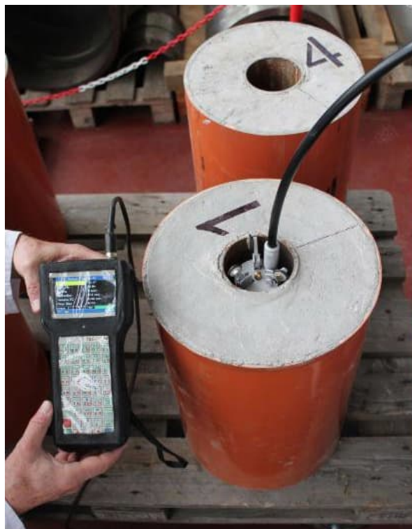
Figure 2. The mock-up of ionization chamber channel surrounded by concrete with various types of defects.
