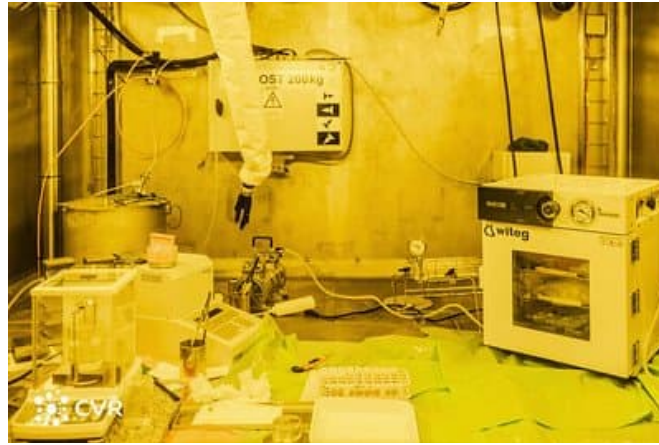
Figure 9. Water and helium pycnometry measurement device in the hot cell
