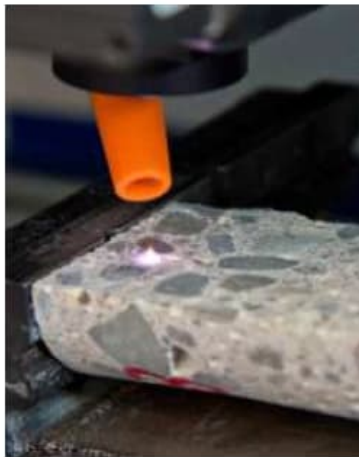
Figure 2. Left: concrete sample with plasma on the surface. Right: Typical spectrum measured on cement paste in the near-infrared wavelength range. Important peaks are marked by the element symbol.
