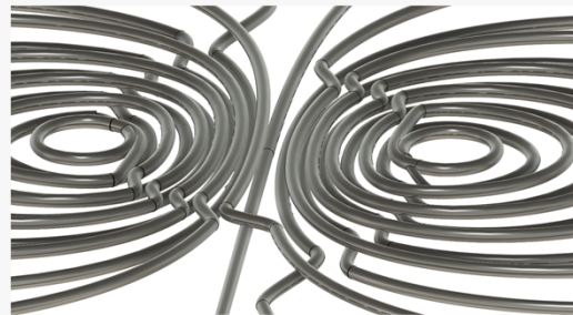
Fig. 3. 3D model of the wire paths in a figure-of-eight coil. The wires were arranged in partially overlapping turns to induce an electric field in the brain with desired voltage, energy, inductance, and electric current requirements.
