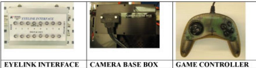
Figure 2: MEG control room components
