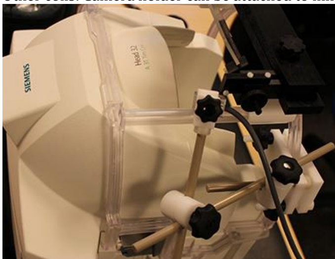
Image 17. Camera holder is attached to the mirror holder
