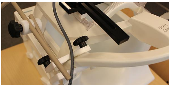
Image 16. Camera holder is attached to the coil directly
