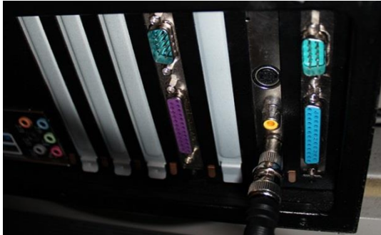
Image 11. EEG PC from the back. Coaxial video cable is attached to the frame grabber card.
