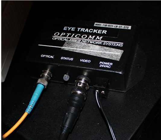
Image 10. Cables from left to right: optical fiber, coaxial video cable and power cord.
