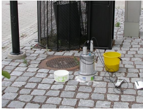
Picture 3. Portable chamber system with infrared carbon dioxide analyser and temperature and relative humidity probe for soil CO 2 flux measurement. Image by Anu Riikonen.
