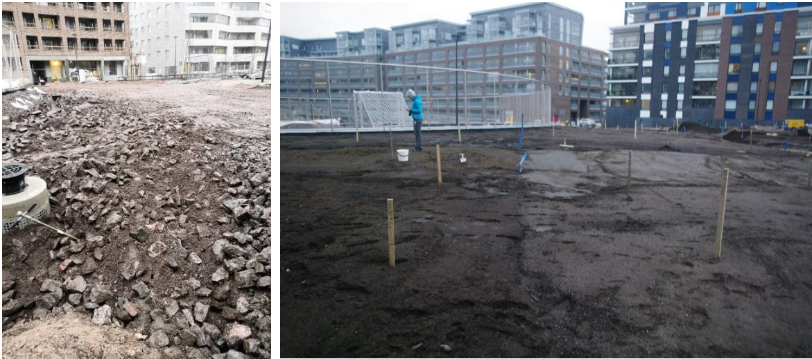
Picture 2. Soil sampling at the Jätkäsaari demonstration site in November-December 2019 while the park was under construction. Left: structural soil, right: planting soil. Images by Päivi Soronen and Priit Tammeorg.
