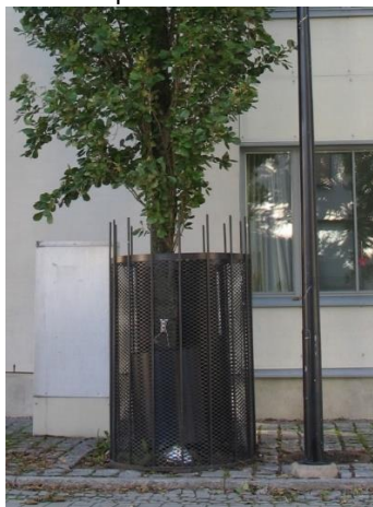
Picture 4. Sensors installed on urban tree trunks can be protected by surrounding the entire tree base in custom made steel mesh cage. Image by Anu Riikonen.
