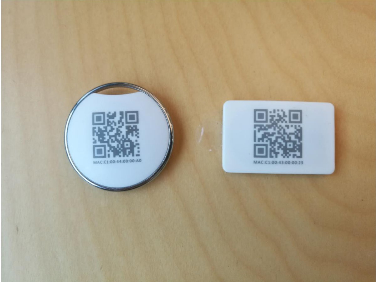
Figure 4: Two types of beacons used in iCONS.
