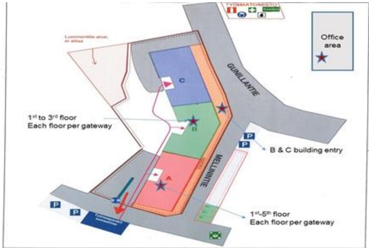
Figure 22. Skanska case study gateway placement floor plan
