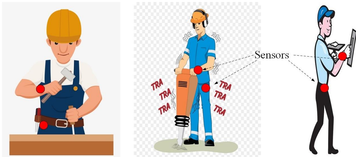
Figure 9: Beacons with accelerometer sensors used by the workers for activity recognition.
