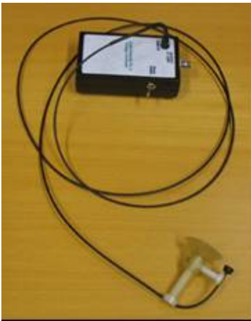
Image 3: Light to voltage converter
