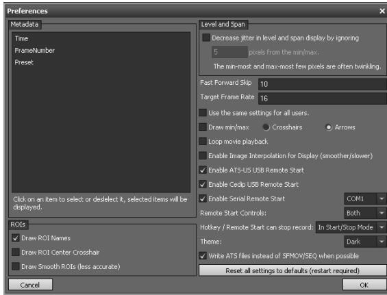
Recording starts when TTL pulse is sent from the parallel port of external PC (Stimulus PC, COM1). For example you can use *Presentation* software to do this.
