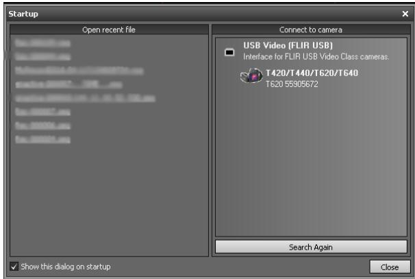
Click available device on the “Connect to camera” -panel. Software connects to the camera and live video should be visible.
