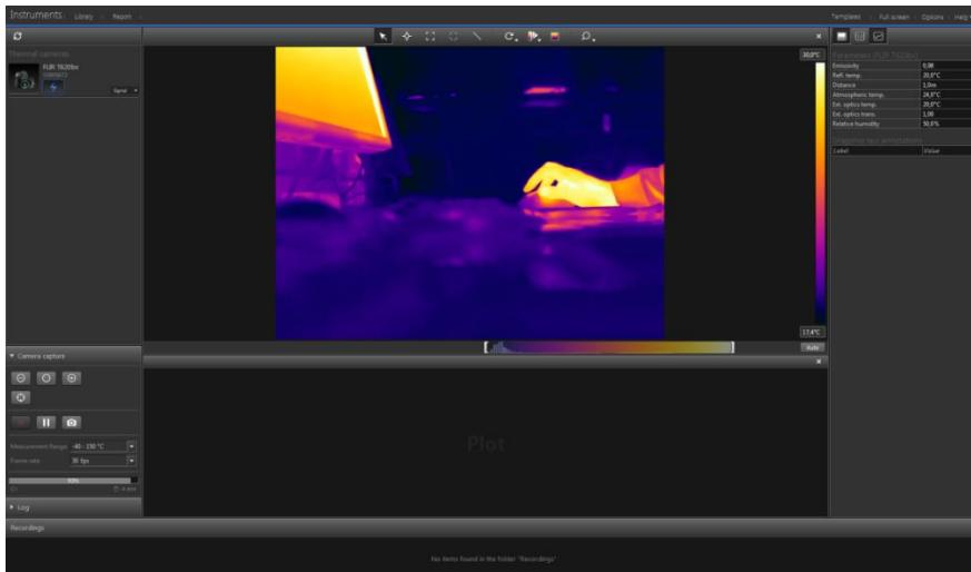
Camera can be controlled from the “Camera control” panel (focus, color adjustments, taking snapshots). Video recording option is only available in licensed or trial versions.
