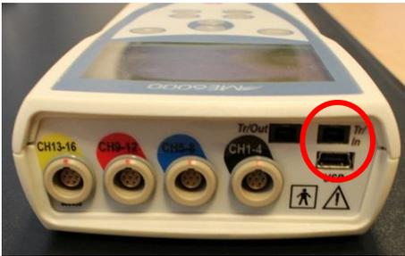
Triggers will show as flags in on-line monitoring viewing window, or they can be seen in the data file as “markers”.
