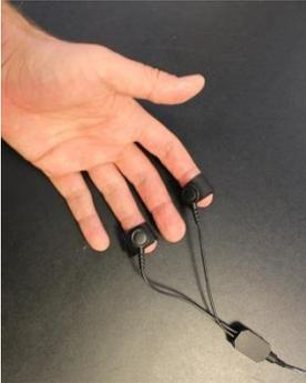
Cleaning: After the use, clean the sensor using a water and mild soap with dampened cloth.
