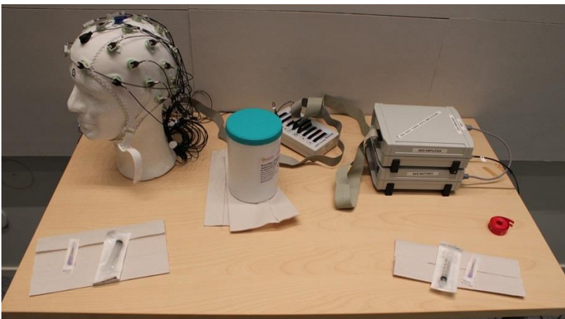
Image 9: Preparation table ready for preparation. ActiCap on the top left, control box in the top middle and amplifier and power pack on the top right. Consumer products for two are in the bottom, including needles, syringes and pack of Gel. Also some paper towels to wipe things. Red measurement tape is on the right.
