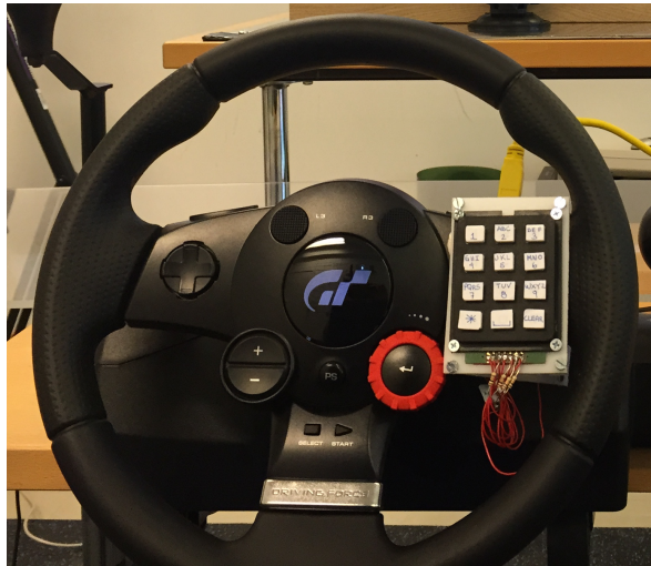
Figure 2. Prototype design of the T9 integrated to the steering wheel, which was used in the evaluation study.
