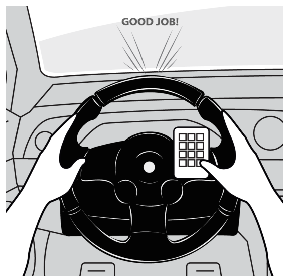
Figure 1. T9+HUD combines a physical 3x4 keypad on the steering wheel with a head-up-display (HUD) for projecting output on the windshield.
