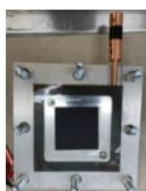
Standard single Fuel Cell made at Aalto (squared shape)
