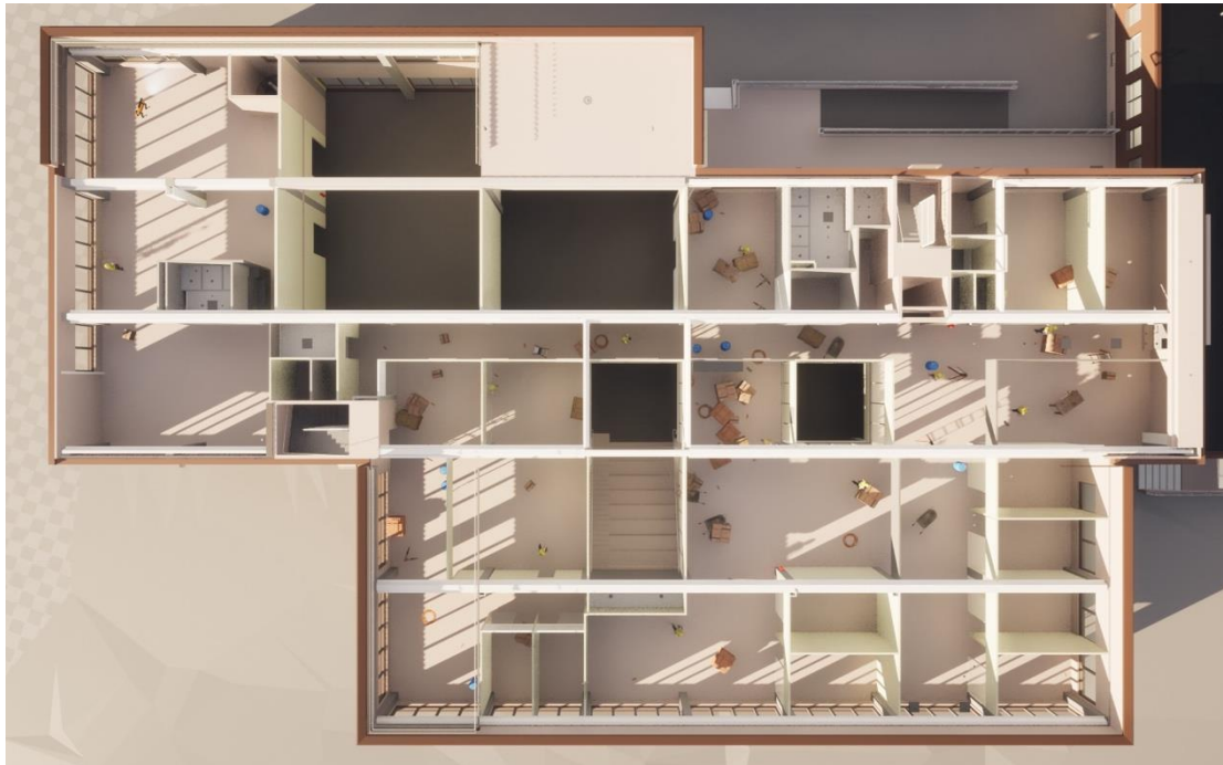
Figure 6: Unreal Engine-based simulation for testing navigation in the presence of various obstacles
