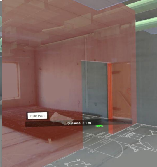
Figure 30. Virtual drywall, floorplan and building services engineering 3D models perceived through AR glasses, as if part of the real world
