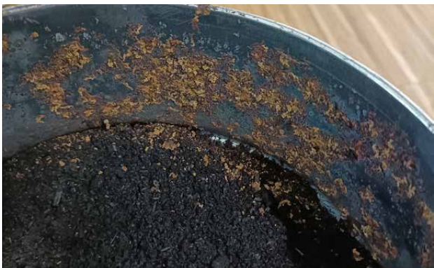
Figure 7 The metallic sample container reacted with the biochar made from soft green waste, showing corrosion (top right) and peculiar protruding crystalization on the metal bucket surface (top left)
