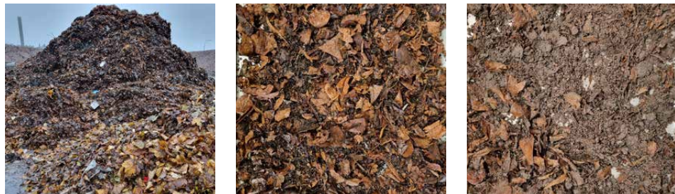
Figure 8 Street sweeping sample variations from lower (bottom center) and higher (bottom right) sand and gravel content. The material piles (bottom left) also contained considerable amounts of garbage (eg. coffee cups, candy wrappers) which were not included in the samples
