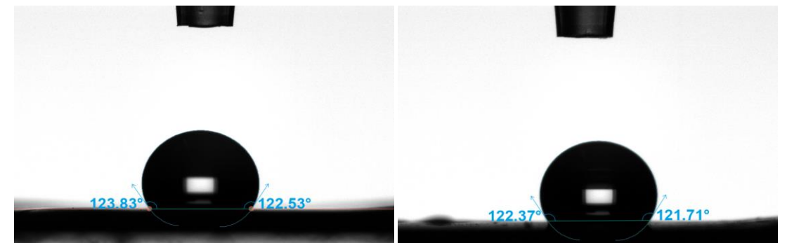
Contact angle of (a) virgin and (b) fouled membranes.
