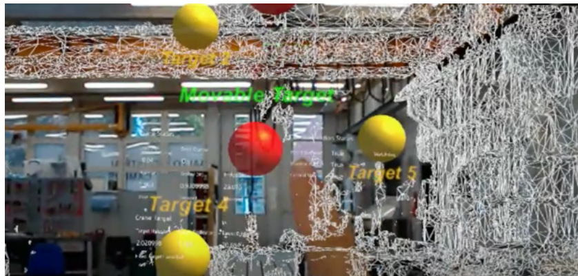
HoloLens View During Movable Target Control (with Spatial Mapping)
