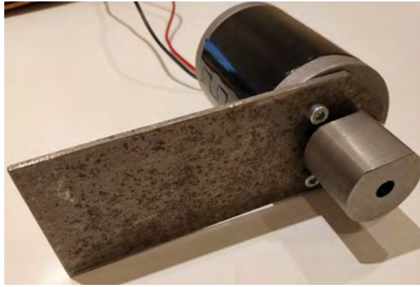
Figure 5. Vibration motor assembly, with a DC motor, steel mounting bracket and an eccentric weight installed to its shaft.
