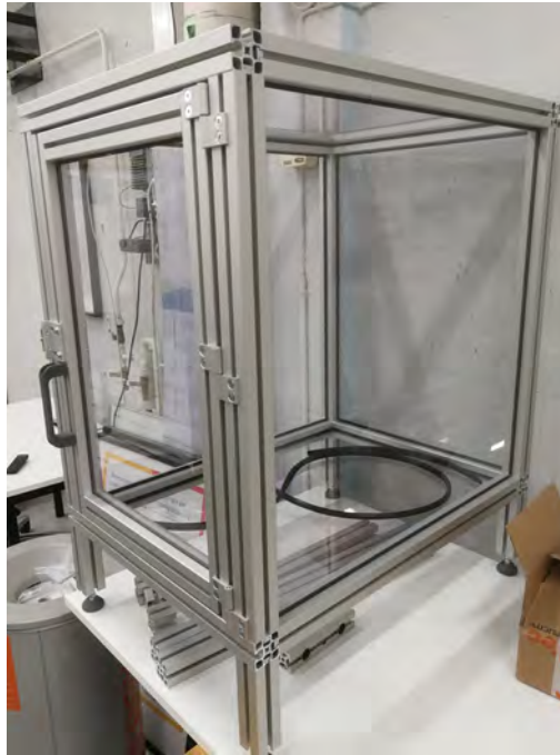
Figure 4. The frame with airtight chamber for the device.
