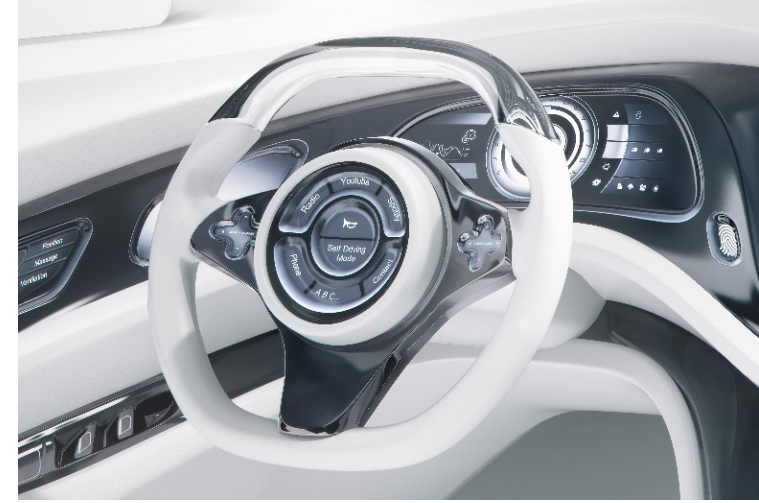
Smart Steering wheel with touch and heating integration
