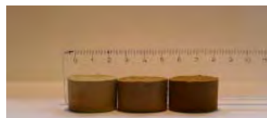
Figure. The photo shows the foams after removal of the top layer in their original state. Notice the increase in color as particle content increases from 2.5 wt% to 10 wt% (from left to right).
