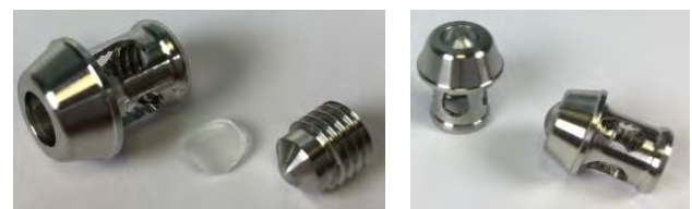
Figure 2. Left: Adapter with urinary catheter specimen and grub screw. Right: Urinary catheter specimen fixed in the adapter.
