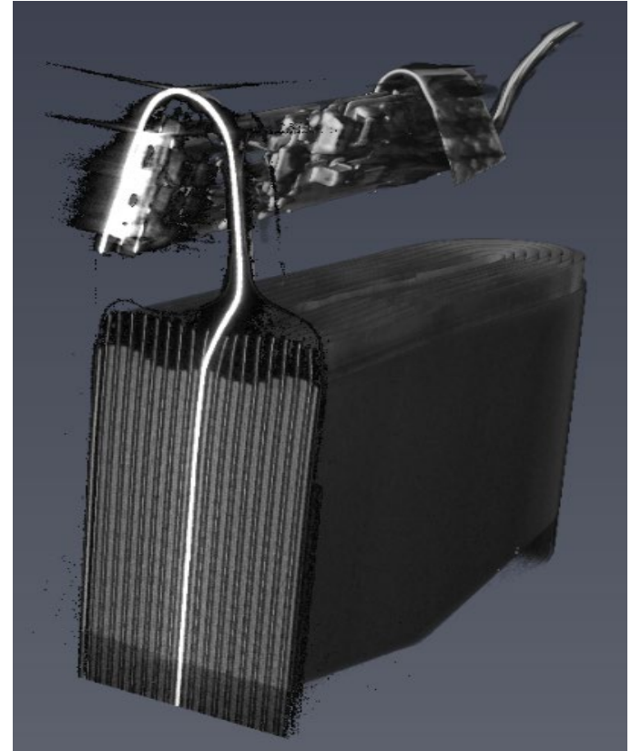
XCT Shadowgrams at 10 \mu\text{m} res. 500 mAh LiPo cell
