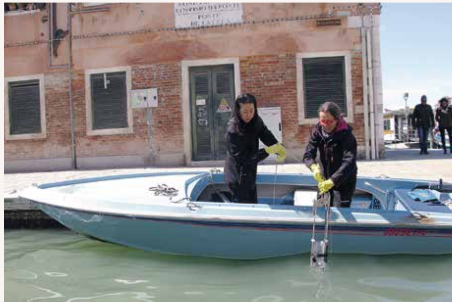
Sediment sampling in the historical centre of Venice with the Limnos sampler provided by the Finnish Environmental Institute SYKE. Image: Pauliina Purhonen
